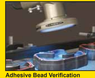
Adhesive Bead Verification
