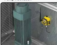
A Banner Wireless Node, is used to activate a pump that could be used for direct irrigation or to fill a tank. If the radio link is lost for any reason, the Node outputs can be configured to stop automatically and send an alarm to key personnel.
