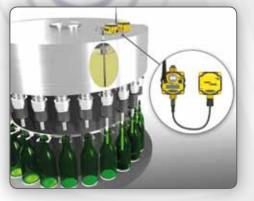
Replace slip rings with on-board Wireless monitoring of level, pressure and temperature
