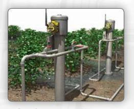
Irrigation Control system pressure, solenoid valve activation and counter input on a Wireless Node optimised for battery-power
