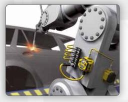
Robot equipment Avoid costly shutdowns caused by broken cables via wireless data transfer from a moving robotic arm to the control panel
