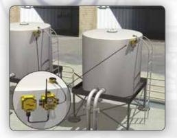
Tank Level Monitoring Measure liquid level and activate a pump or open a valve with a Wireless FlexPower Node
